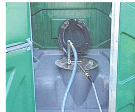
To clean the interior, the system is connected to existing water and vacuum lines. The cleaning machine is attached to a vertical support stand and placed into the unit. The door is closed and the pump turned on. Within the confines of the unit, the powerful rotating spray cleans up to 95% of the unit's interior surfaces includ-
